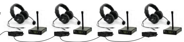
The first Monitoring Unit receives the main feed from the sound system or directly from any existing microphone. In turn, each additional Monitoring Unit daisy-chains to the next Monitoring Unit with a standard XLR>XLR cable to share the main feed with as many Monitoring Units as your application calls for. Each interpreter's headset plugs into their corresponding Monitoring Unit.
