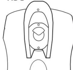
For hands free operation of the R35-8 receiver, use the provided belt clip to secure the unit on your belt, pocket or pants.
